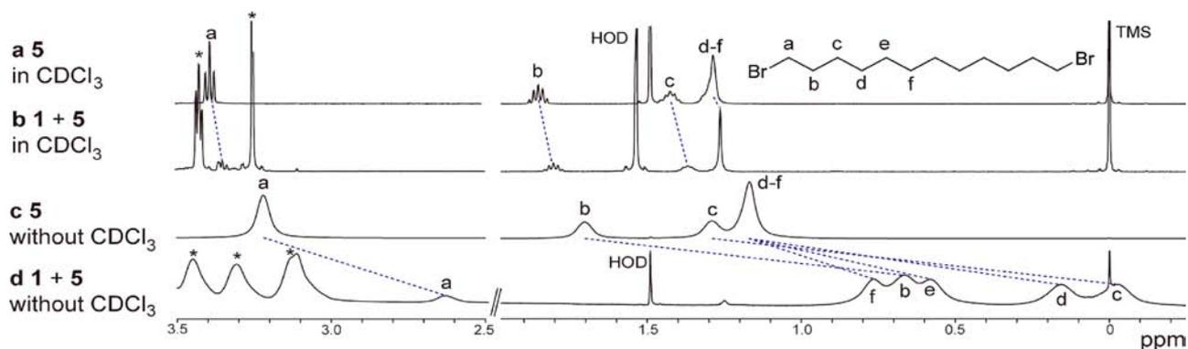
**Figure 2.**  $^1\text{H}$  NMR spectra at 42 °C. (a) **5** (1 mM) in  $\text{CDCl}_3$ , (b) 1:1 mixture of **1** (1 mM) and **5** (1 mM) in  $\text{CDCl}_3$ , (c) **5** without  $\text{CDCl}_3$ , and (d) equimolar mixture of **1** and **5** without  $\text{CDCl}_3$ . Peaks with asterisk are proton resonances from **1**.
