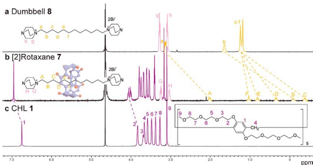
**Figure 4.**  $^1\text{H}$  NMR spectra of (a) dumbbell 8, (b) [2]rotaxane 7, and (c) CHL 1 in  $\text{CDCl}_3$  at  $25^\circ\text{C}$ .
