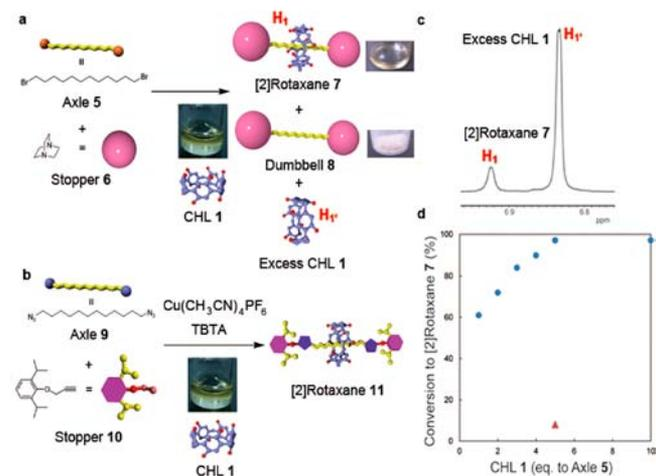
**Figure 3.** Synthesis of [2]rotaxanes by (a) cationization and (b) Huisgen reaction. (c) Partial  $^1\text{H}$  NMR spectrum ( $\text{CDCl}_3$ , 25 °C) of the mixture after the reaction of axle **5** and stopper **6** in CHL **1**. (d) Percentage conversion to [2]rotaxane **7** versus molar equivalents of CHL **1** compared to axle **5** in the CHL systems (blue circles) and in the typical solvent system (brown triangle).
